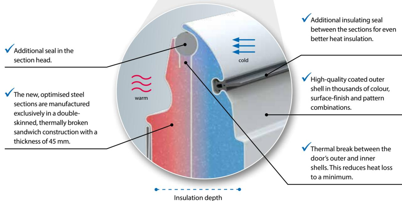
✓ Additional insulating seal between the sections for even better heat insulation.
